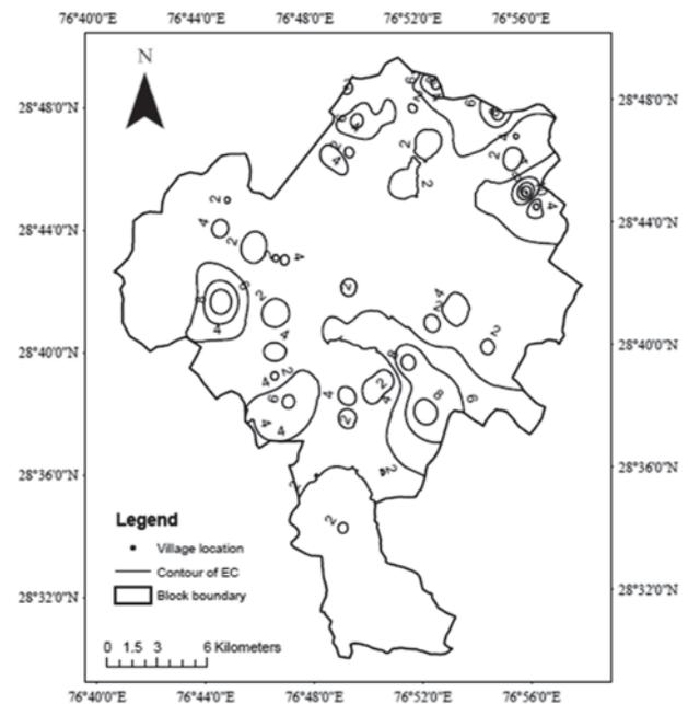
Fig. 3. Contour map of EC of groundwater in Bahadurgarh block
