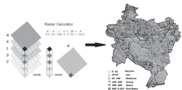
Fig. 8. Soil loss prediction process for Sakarya Basin
